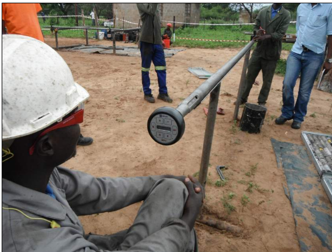
Figure 9-3: Drill core orientation marking (Source: SRK site visit, 2014).
