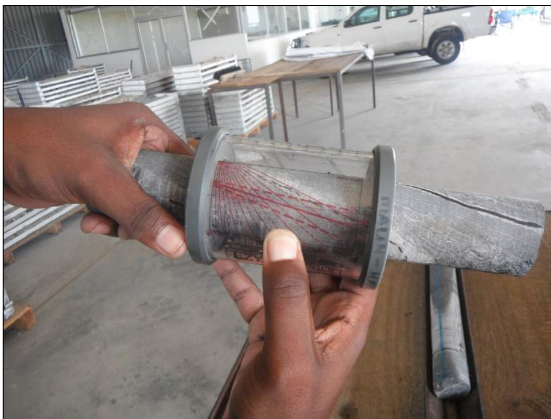
Figure 10-1: Structural core logging using EZY-Logger Goniometer (Source: SRK site visit, 2014)
