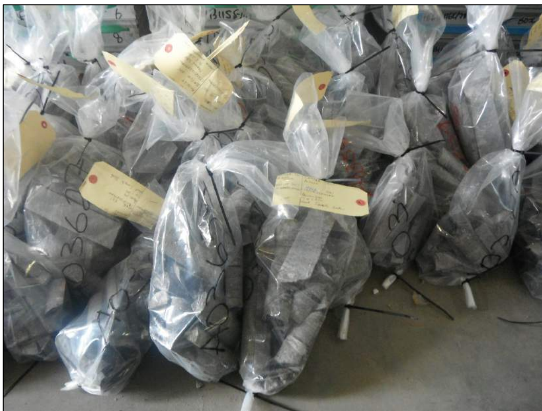
Figure 10-5: Half-core samples bagged and tagged by Gcwihaba (Source: SRK site visit, 2014)
