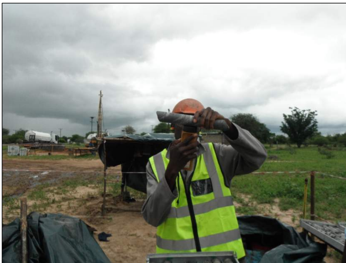
Figure 10-2: Magnetic susceptibility measurement at the drill rig (SRK site visit, 2014)
