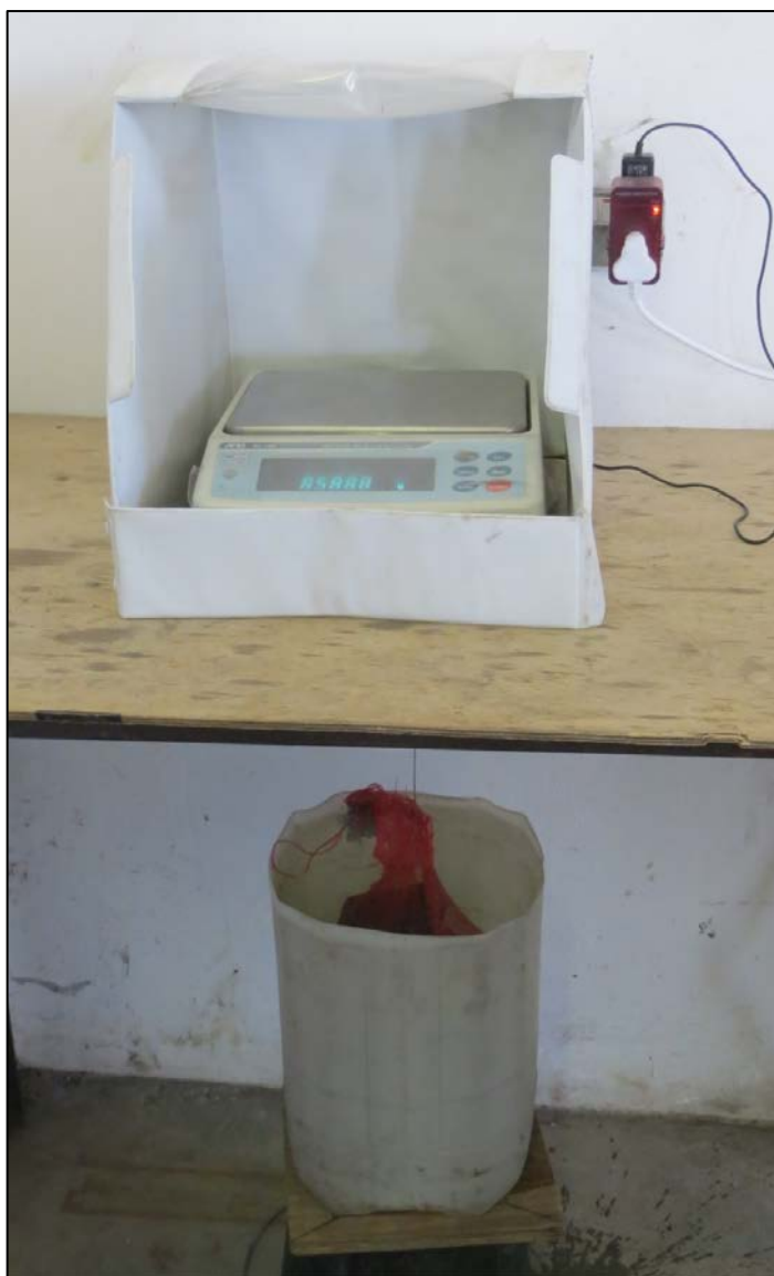
Figure 10-3: Density measurement equipment (Source: Gcwihaba protocols, 2014)
