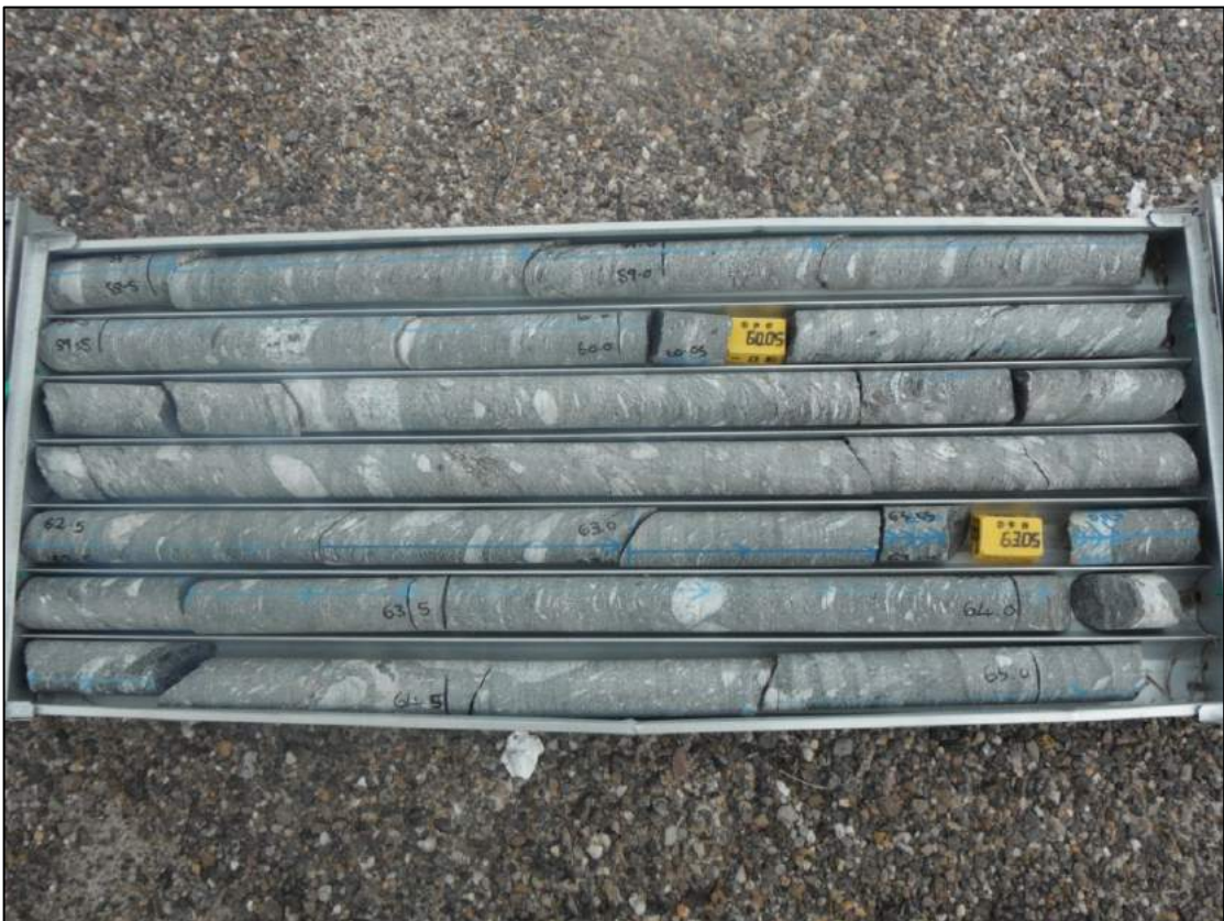
Figure 6-13: Diamictite Schist - geodomain DIA (Source: SRK site visit, 2014).
