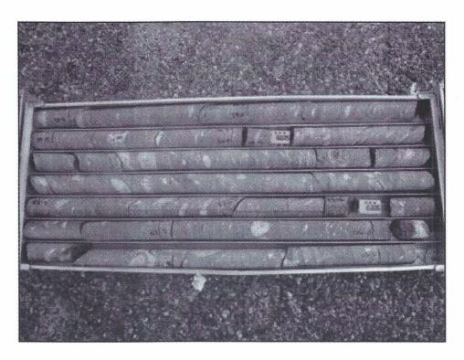
Figure 4-4: Diamictite Schist - geodomain DIA (Source: SRK site visit, 2014).
